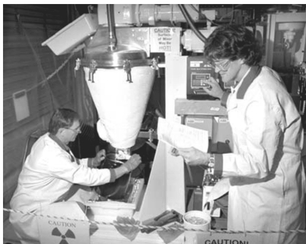
FIGURE 6.3.2 Pilot-scale process equipment for Sulfur Polymer Stabilization/Solidification (SPSS) treatment of mercury waste.
