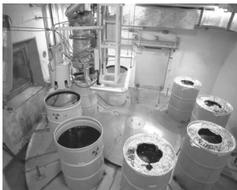
FIGURE 5.3 Bitumen wiped film evaporator system installed within a hot cell at the Korean Atomic Energy Research Institute.
