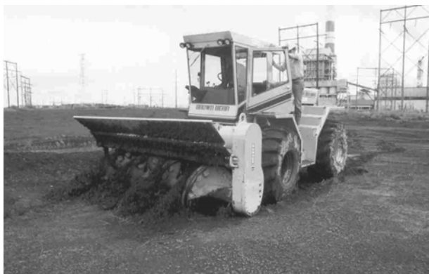
FIGURE 13.6 In situ mixing with a tractor-mounted disk harrow.
